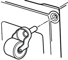
3. Screw casters into dryer base at four corners and tighten securely.
