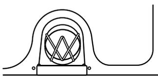
2. Install exhaust hood. Use caulking compound to seal exterior wall opening around exhaust hood.
