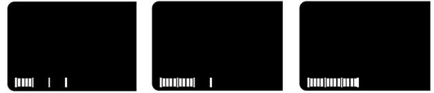
The progress bar is a visual picture of the estimated running time of a cooking cycle. It will appear during Cook, Defrost, Reheat and Sensor functions. The lines in each of the segments will light from left to right as the time nears the end. When all 12 lines (all 3 segments) are lit, the cooking cycle is complete.
