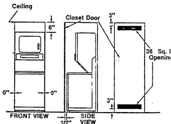
Each opening area must have a minimum of 36 square inches. These openings must not be obstructed. (Louvered door with equivalent air opening is acceptable).
