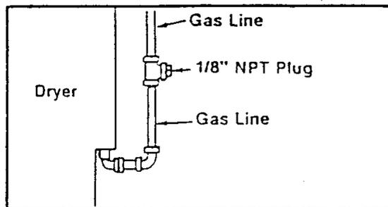
The gas supply should be connected to the dryer using pipe joint compound or a Teflon tape on male thread connections. **NOTE:** Any pipe joint compound used must be resistant to the action of any liquefied petroleum gas.
