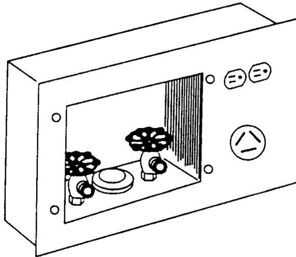
If the faucets and/or drain is located to either side of the stacked washer/dryer, openings are located in the dryer stand uprights to allow hoses and power cords to be passed through. This is to allow installation against the back wall. (This is dependent on venting used.)
